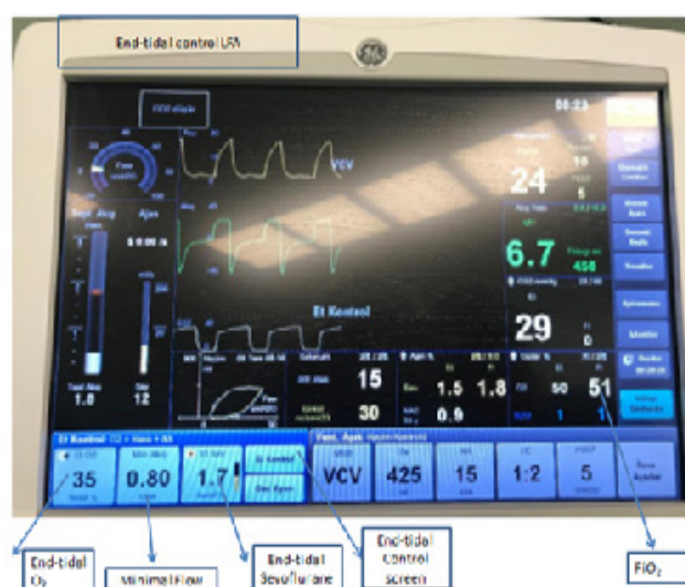
Figure 2. After the increase in the flow rate and in FiO 2 (long time), the flow rate is decreased at 800 ml/min (end-tidal controlled LFA).
